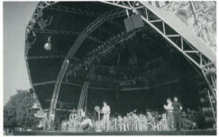
The lights' layout for the stage was dictated by the D-shaped truss and featured Pars, Fresnels, and 22 Vari*Lites.
